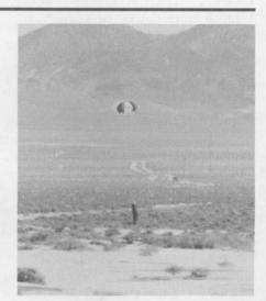
PARACHUTE RECOVERY SYSTEM to soft-recover artillery projectiles fired from 155mm howitzers has demonstrated increased reliability, compared to its predecessor, in all 15 of its tests to date. The test shown here was at Tonopah Test Range.
